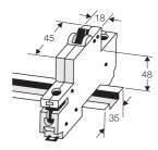
Dimensions according to DIN 43880 for DIN rail mounted device
