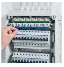
Note to Mi Circuit breaker boxes: Spare equipment openings in protection covers are to be covered with blanking strips to prevent accidental contact (blanking strips are enclosed for 50 % of equipment openings) Dimension of 1 module: 1 Module = 18 mm
