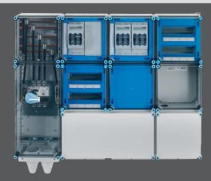
Combinable enclosure system, insulation-enclosed, total insulated, degree of protection IP 65, for the assembly of power switchgear and controlgear assemblies (PSC) up to 630 A in accordance with IEC 61439-2.
